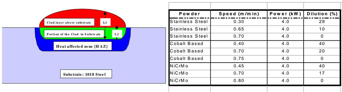
**Figure 3: Standard visual measurement of dilution was performed through the equation  $L2/L1$ .**
