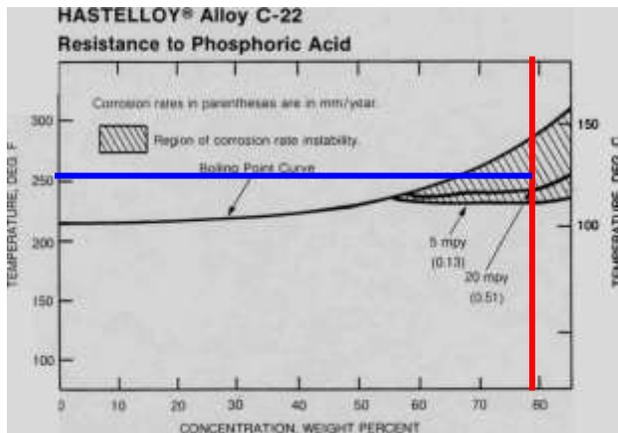
**Figure 9: Iso-corrosion diagram for the C22 alloy as well as the mass loss for each sample.**
