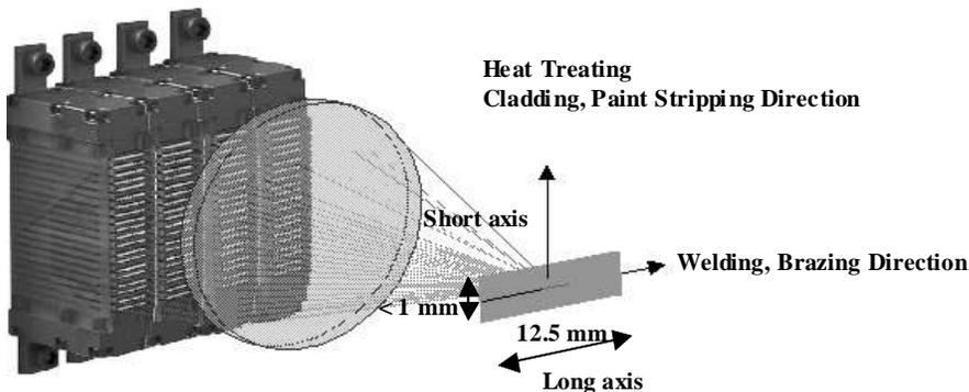
**Figure 1 – Focus Configuration of Line Source HPLLD**
