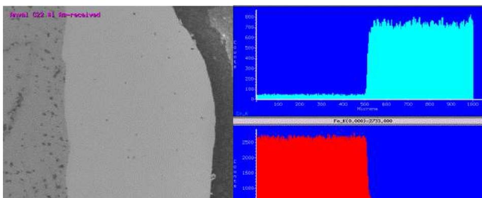
**Figure 6: A SEM line trace of a NiCrMo clad produced at 0.45 m/min, 4 kW.**
