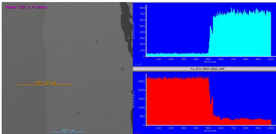
**Figure 7: SEM line trace of overlapping passes of NiCrMo alloy produced at 0.7 m/min, 4 kW.**
