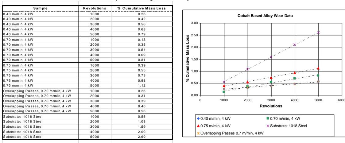
**Figure 10: Pin on Disk wear test results.**
